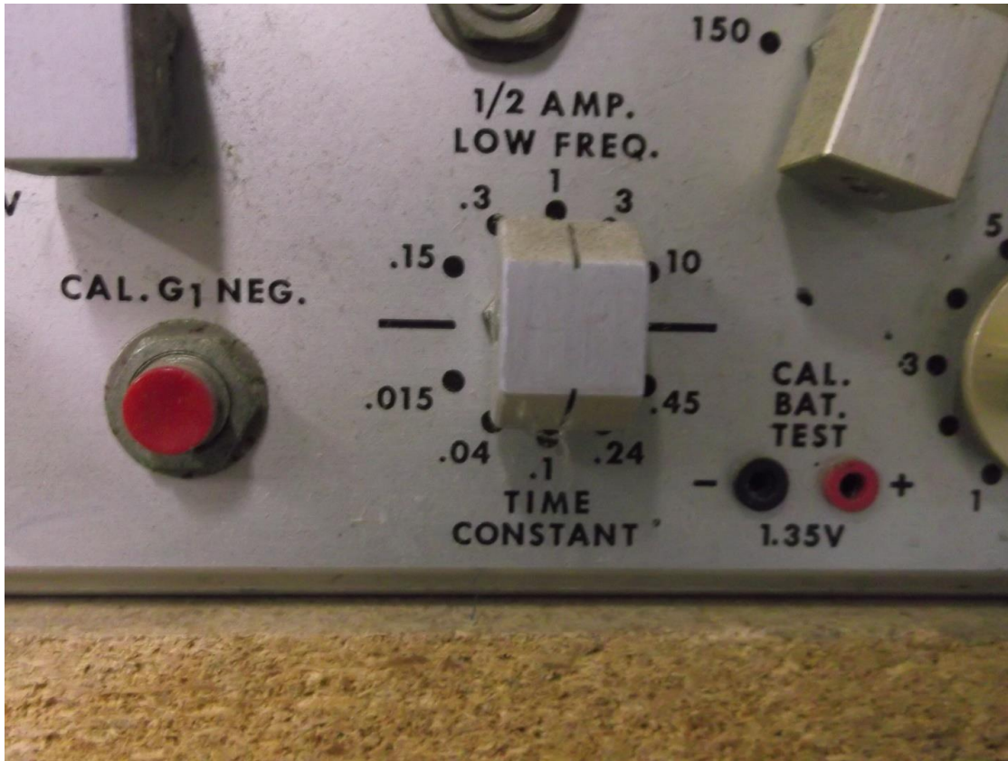
Figure 3. Grass EEG amplifier showing combined “low frequency / time-constant” control, illustrating the interdependence of these two settings.
